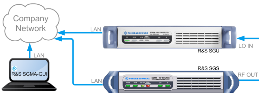
Fig. 5-5: Connection of an R&S SGS and an R&S SGU in a company network
